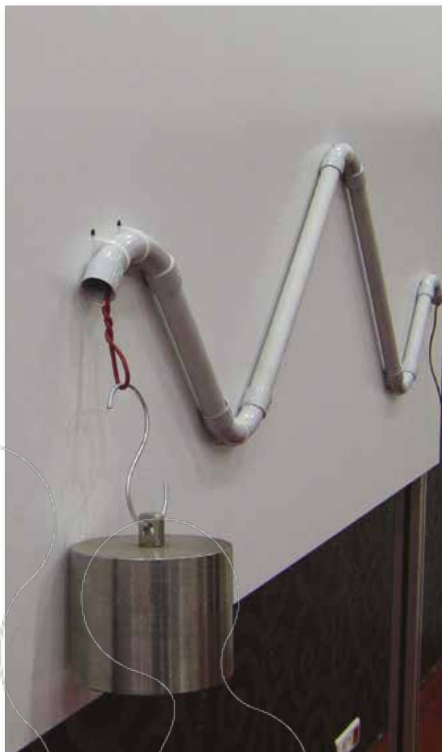
Slick cables can move through ducts even with small amount of force.
