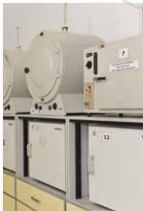
Ovens used for aging tests.
