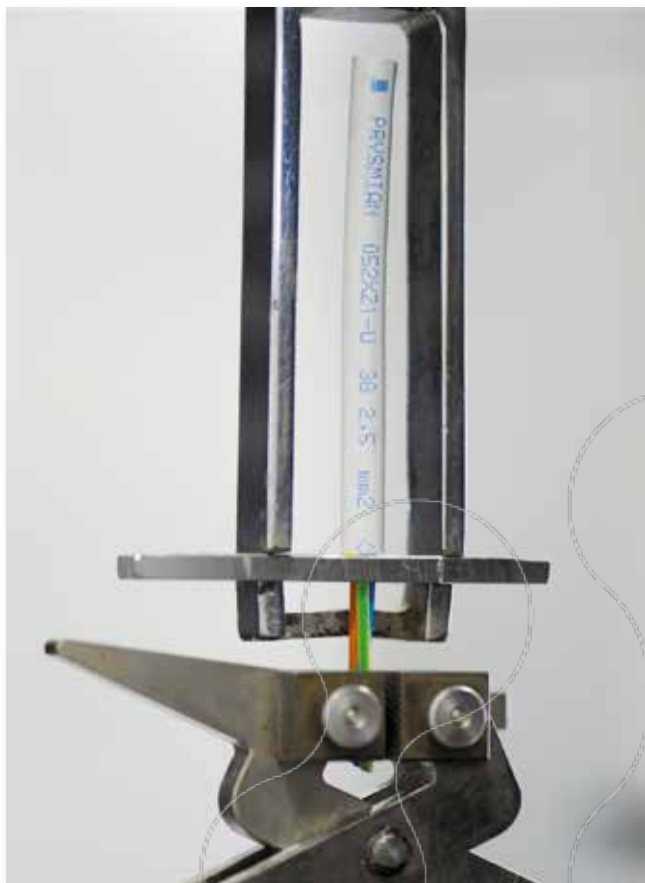
A cable sample in the stripping test.
