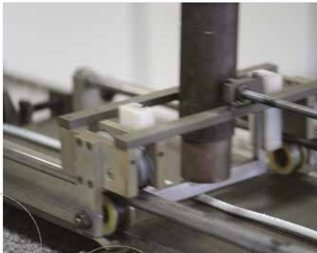
A cable sample in the abrasion test.
