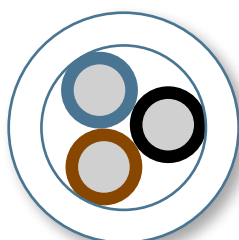
Outer jacket wall thickness cross-sectional view.
