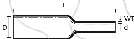
Heat Shrinkable Tubing 3:1 with adhesive
