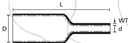
Heat Shrinkable Tubing 4:1 with adhesive
