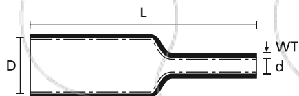
Heat Shrinkable Tubing 3.5:1 with adhesive
