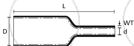
Heat Shrinkable Tubing 4:1 with adhesive.
