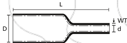
Heat Shrinkable Tubing 4:1 with adhesive
