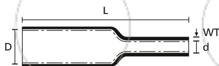
Heat Shrinkable Tubing 3:1 with adhesive
