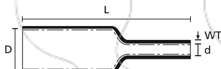
Heat Shrinkable Tubing 3.5:1 with adhesive
