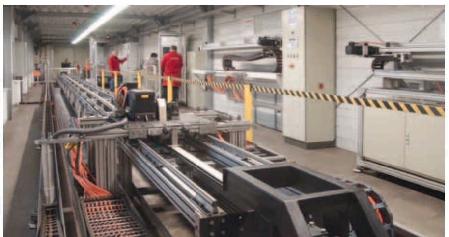
Drag chain test system
