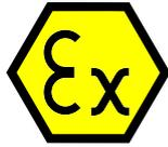
Ex ib e IIC T2..T4 Gb
