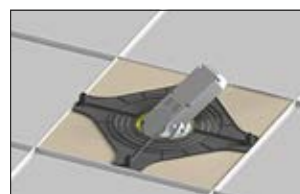
3. Insert the downlight through the cutted hole.
