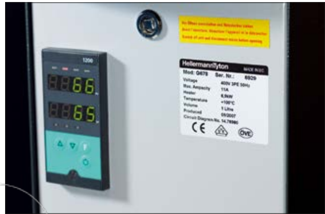
Professional type plate on a heating unit.
