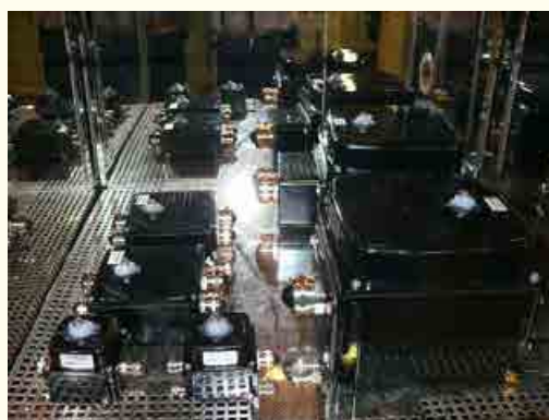
Picture 21: example of conditioning in climatic chamber
