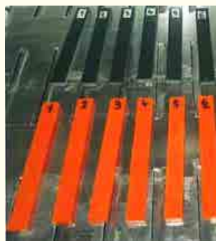
Picture 26: examples of samples for testing the resistance to ultraviolet light
